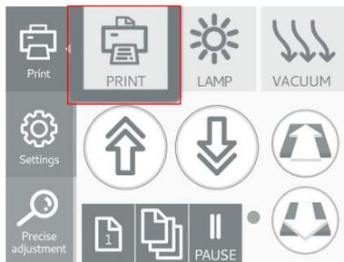
5. Go back to azon utility software and from it start nozzlecheck. After RIP or driver installation nozzle check can be done from both (if printing from RIP or driver USB cable is not needed)
