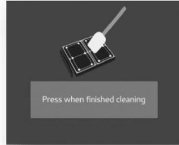
**3.** Dip the foam swab in to print Cleaning Liquid. Do not double dip , this will contaminate the entire bottle. Once the swab is completely dirty dispose of it properly. Only use lint-free cleaning foam swab provided from Azonprinter company . If you use cotton swab or something similar the cotton fibers will clog the print head.
